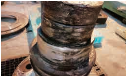
OUTBOARD 軸心磨損
