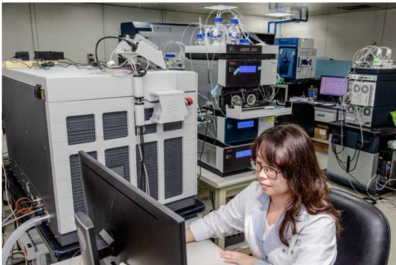
..... Molecular Medicine Research Center- Orbitrap Fusion Lumos Tribrid Mass Spectrometer
