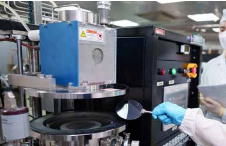
High density plasma etching for microstructures on Si wafer
