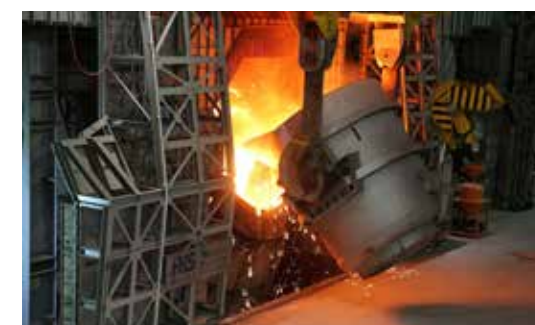
Hot metal charged into converter(BOF) and blowing on 1 st Jun 2017.
